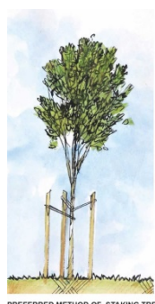
Figure 17.2 Preferred method of staking trees
